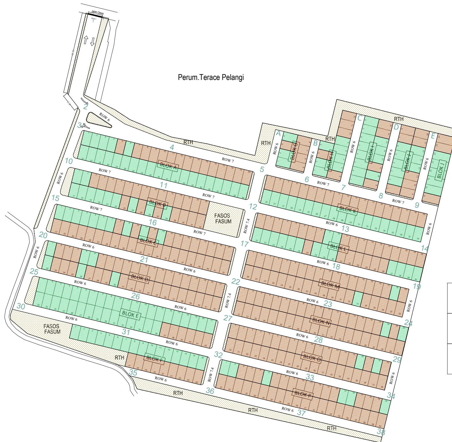
MAPING CUTNFILL KAVLING SCALE 1 : 1500
